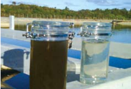
Influent (left) vs. effluent (right)
