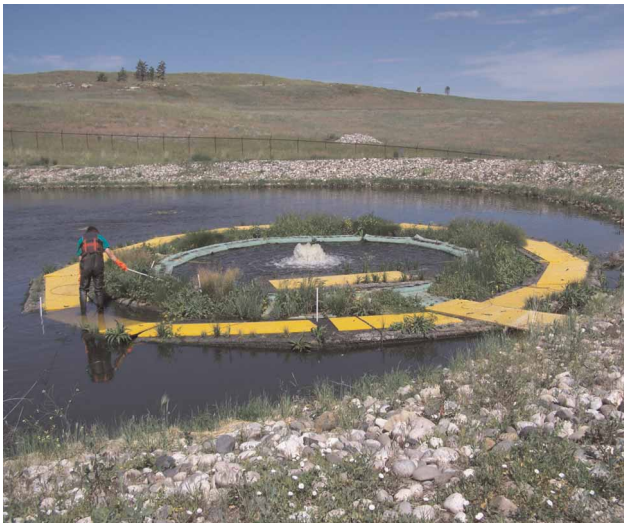
Figure 1 | A 232 m 2 FTW in an aerated lagoon at Rehberg Ranch Subdivision, Billings, MT USA. The FTW is circular, with a radial fountain pump installed in the center. The body of the island is designed to float below the surface in order to maximize constituent uptake by biofilms growing on the plastic matrix. Parameters being tracked include suspended solids, BOD, nitrogen and phosphorus. The island was installed by Headwaters Floating Island, LLC during November 2009, and planted during the spring of 2010. Periodic water quality testing is being provided by the City of Billings, MT and Floating Island International, LLC.
