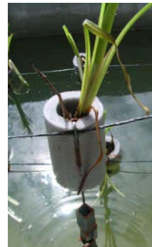
Figure 5. Plants supported at the water surface by cables suspended across the pond (source: LIFE02 ENV/E/182, 2005).
